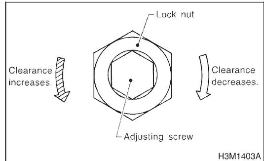
2) In case of the occurrence of problems 1. and 4. mentioned previously, perform the adjustment as follows: Adjusting procedure: Tighten adjust screw to 9 N·m (0.9 kg·m, 6.5 ft·lb) torque, then back off three turns.
